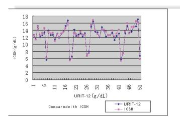
**Precision:** CV<5%,testing samples including high, medium & low concentration, the CV of 10 repeated test results is 1.8%, 2.2%, 2.7% respectively.
